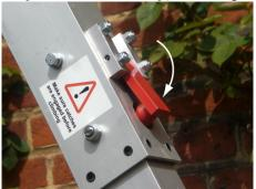
12. Continue winding winch to raise platform until the platform is above the desired height.
